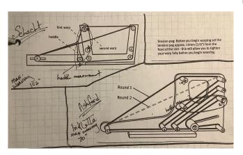
Each brand of Inkle loom has it's own warping directions and maximum warp length. By skipping certain pegs, the max warp length may be shortened. Shown below is a short band on the Schacht, long band on the Inklette.
